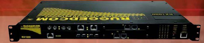
SCADA Cyber Security Appliance
