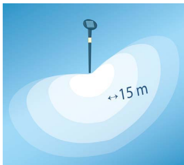
Fig.: Kidneylike cone of light
